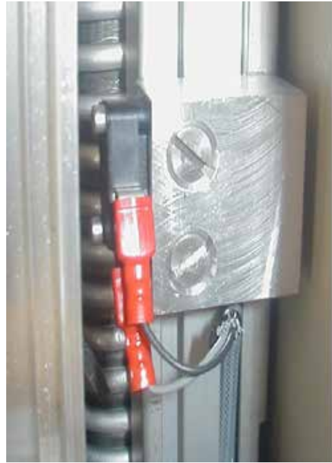
Interior detail, showing part of the spring mechanism and the adjustable end switch for stroke length adjustment..
