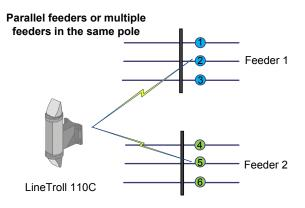
The maximum operating distance between the LineTroll R110C and the indicators is 40m line-of-sight.
