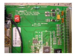
Different types of antennas are available. The default antenna is a 3.3V active antenna, but other types of antennas can be used.'
