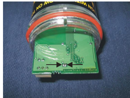
Figure 19. Soldering pads for resetting Battery counter on LT-110E \mu r.
