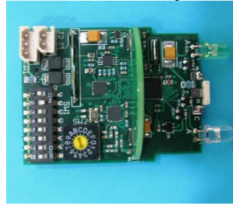
Figure 11b. Rotary switch in location 0009 resetting battery counter on LineTroll 110Tµr.
