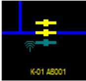
This means there has been a transient fault. The two indicators showing a yellow symbol have most likely clashed into each other, causing the circuit-breaker to trip. The last indicator shows energized line, so the circuit-breaker has restored the feeder upon the reclosing cycle.
