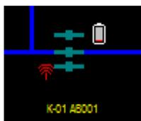
The status of the three indicators shows an energized line with no faults. Low battery from the collector and the communication with one or more indicators are lost are indicated by the two other symbols.
