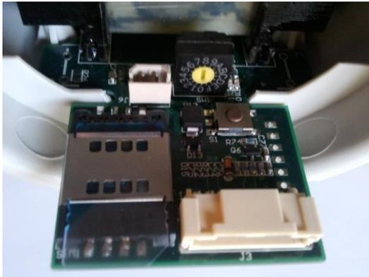
Insert the SIM-card as shown in the picture to the left. The batteries should be disconnected when inserting the SIM card.
