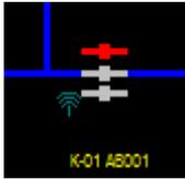
This picture shows a permanent fault on one of the phases. The two other indicators have detected a loss of voltage (de-energized line).
