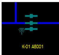
The status of the three indicators shows an energized line with no faults. The indicator and collector batteries are also OK. Symbol for communication between the indicators and the collector shows OK.
